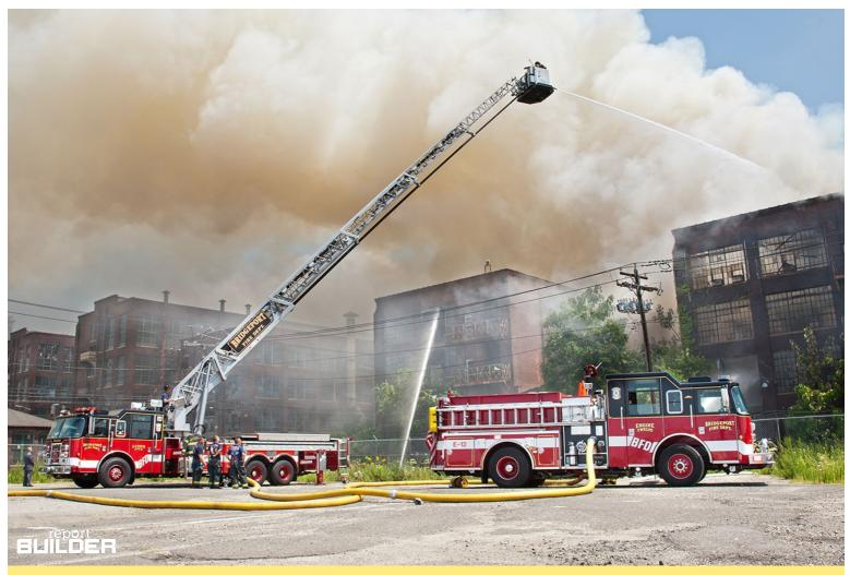
The ladder on this truck allows firefighters to reach high places.
